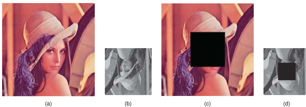
Fig. 7 Cropping test for Varsaki et al.'s 11 method: (a) watermarked image “Lena,” (b) recovery data embedded in (a), (c) when (a) is cropped, and (d) recovery data extracted from the support of the noncropped area.
