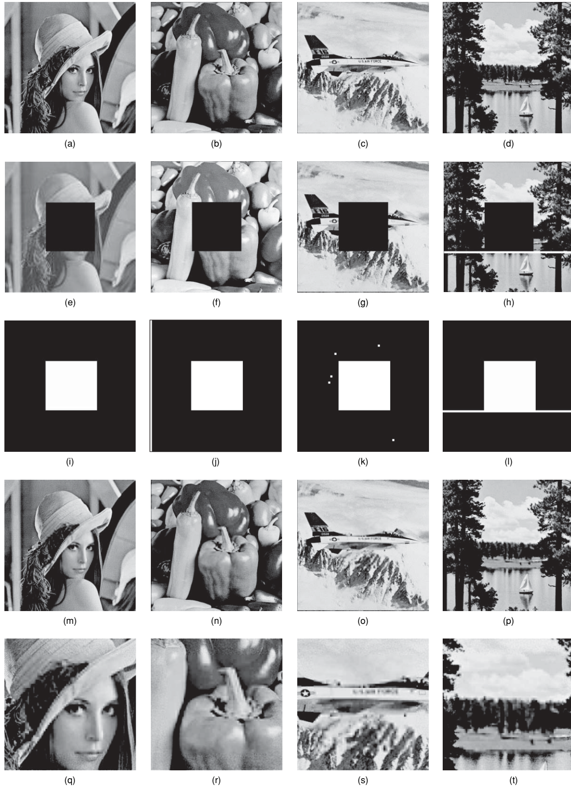
Fig. 3 Robustness test of the proposed method. (a) to (d) our four watermarked images “Lena,” “Peppers,” “Jet,” and “Scenery”; (e) and (f) the four cropped images; (i) to (l) the corresponding verification results, after doing a JPEG compression on (e), adjusting brightness of (f), adding noise to (g), and adding white bar to (h); and (m) to (p) the recovered images; (q) to (t): close-up versions around the recover area of the recovered images (m) to (p).
