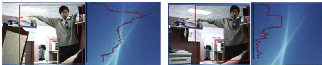
(a) Project Pixels in Bounding Box to Y-axis without Reduction
