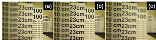
FIG. 4. (Color online) Image performance of the imaging system. The clear image for the objective distance of (a) 300 cm, (b) 23 cm, and (c) 10 cm. See Ref. 15.
