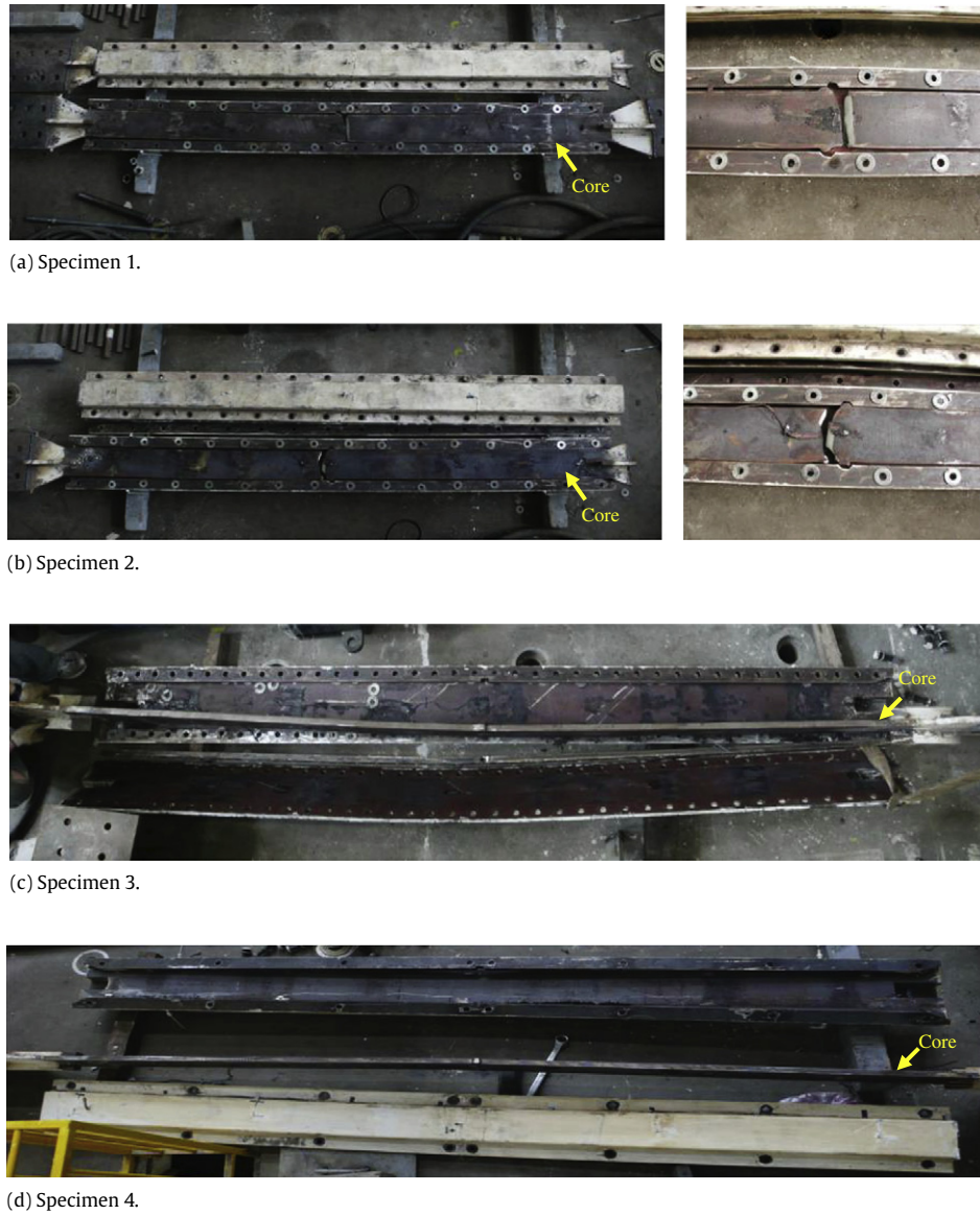
Fig. 6. Failure modes of all specimens after tests.
