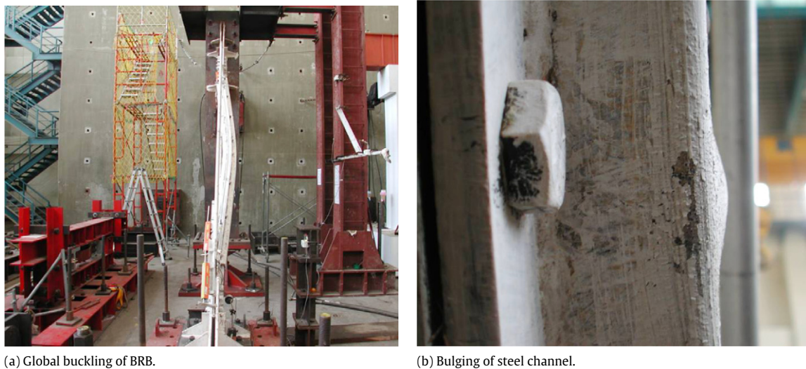
Fig. 8. Specimen 3 observed performance (axial strain of 2.6% during third standard loading test).
