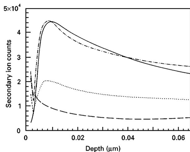
Figure 4 Oxygen depth profile for RIE-etched Si without (—) and with post-etching annealing; (· · · ·) 150 W for 1 h unannealed, (— · —) 50 W for 1 h unannealed, (— — —) 150 W for 1 h, 300 °C for 1 h in N<sub>2</sub>.
