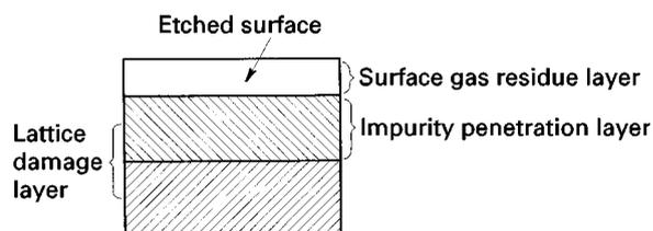
Figure 5 Schematic diagram of RIE-etched substrate.
