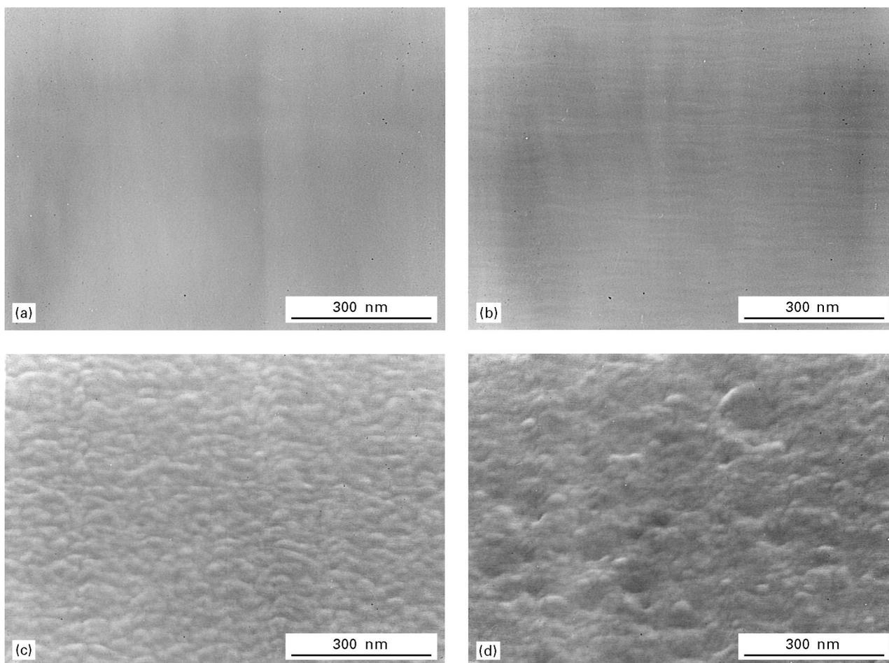
Figure 1 Scanning electron micrographs for Si substrates etched with CF<sub>4</sub> + O<sub>2</sub> for (a) 0 min, (b) 2 min at 50 W, (c) 5 min at 50 W, and (d) 5 min at 150 W.
