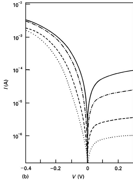
Figure 7 (a)  $I$ - $V$  curves and (b)  $I$ - $V$  curves on semi-logarithmic scale of ITO/p-type Si where Si substrates were etched at 50 W for various times: (—) 30 s, (---) 1 min, (-·-·-) 5 min.
