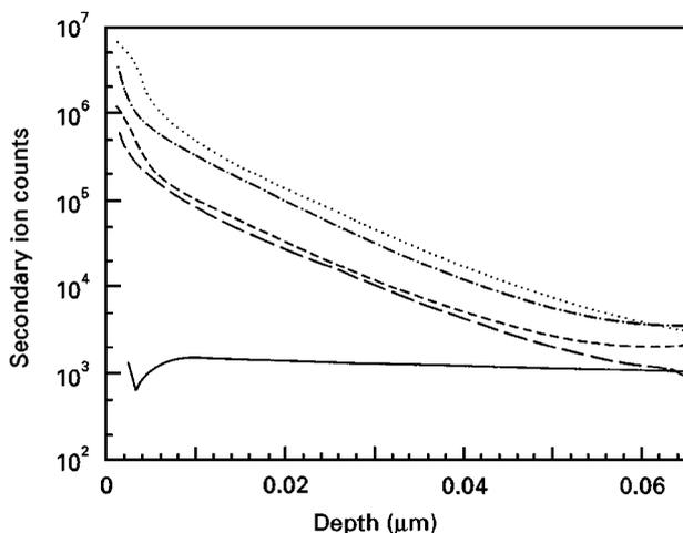
Figure 2 Fluorine depth profiles for RIE-etched Si without (—) and with post-etching annealing (· · · ·) 150 W for 1 h unannealed, (— · —) 50 W for 1 h unannealed, (— — —) 150 W for 1 h, 300 °C for 1 h in N<sub>2</sub>, (— — —) 50 W for 1 h, 300 °C for 1 h in N<sub>2</sub>.
