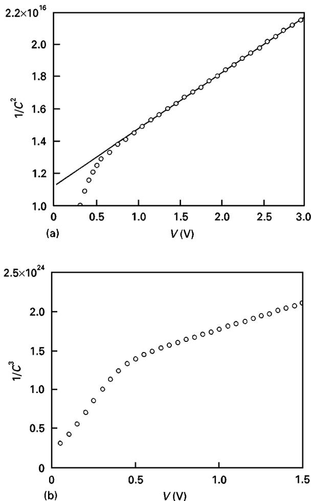
Figure 10 (a)  $1/C^2-V$  and (b)  $1/C^3-V$  characteristics of ITO/p-Si junction where Si substrate was subjected to reactive ion etching.
