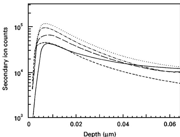
Figure 3 Carbon depth profile for RIE-etched Si without (—) and with post-etching annealing; (· · · ·) 150 W for 1 h unannealed, (— · —) 50 W for 1 h unannealed, (— — —) 150 W for 1 h, 300 °C for 1 h in N<sub>2</sub>, (— — —) 50 W for 1 h, 300 °C for 1 h in N<sub>2</sub>.
