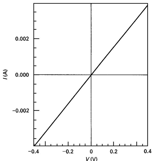
Figure 6  $I$ - $V$  characteristics of r.f. sputtered ITO on unetched p-type Si wafer.
