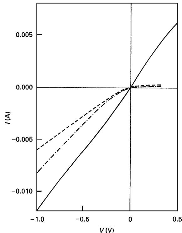
Figure 11  $I-V$  curves of ITO/etched p-Si annealed in  $N_2$  atmosphere at  $300^\circ\text{C}$  for various times; (---) 10 min, (- - -) 20 min, (—) 1 h.
