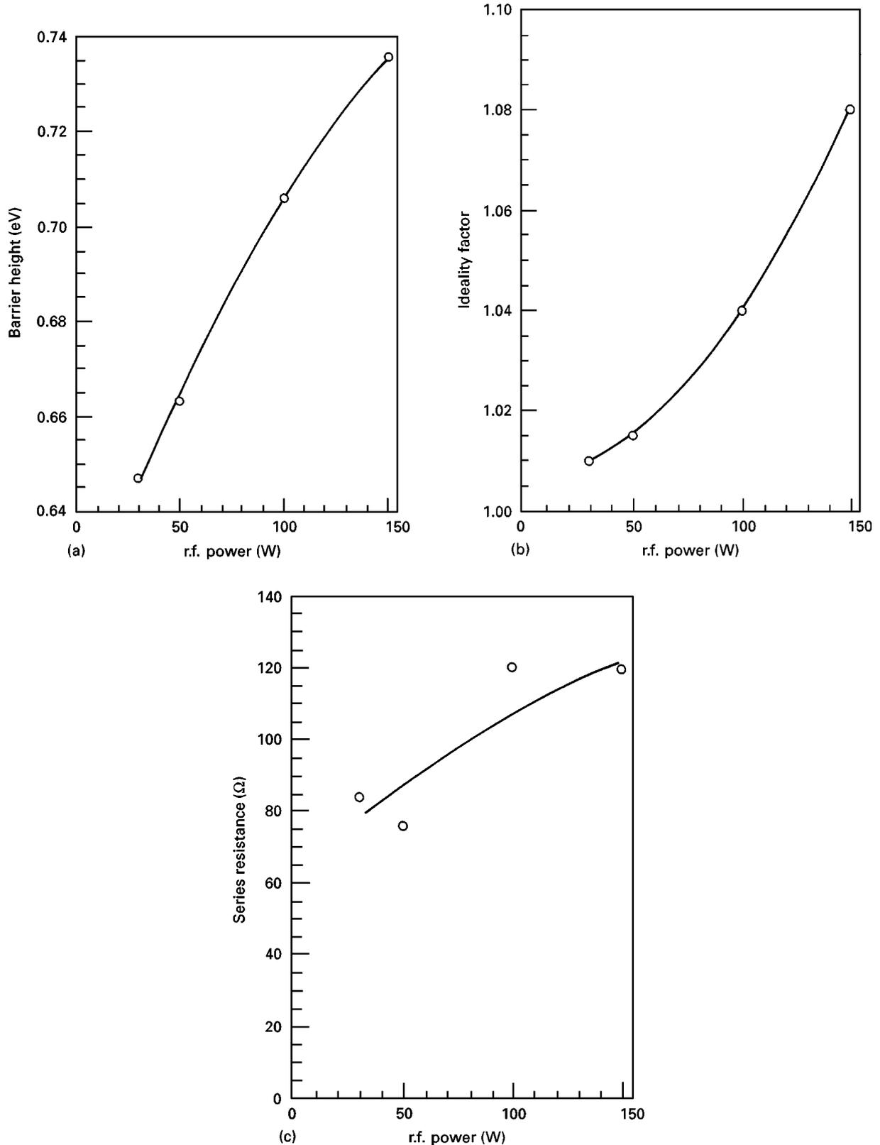
Figure 9 (a) Barrier height, (b) ideality factor, and (c) series resistance of ITO/p-type Si junctions where silicon substrates were subjected to reactive ion etching for 3 min at various powers.
