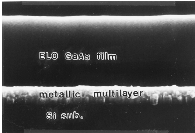
Fig. 5. SEM photograph of a bonded ELO n-GaAs /Pd/Ge/Pd/n + -Si sample.
