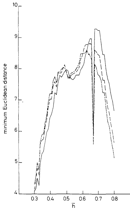
Fig. 2 Minimum Euclidean distances against averaged modulation index \bar{h} for asymmetric MHPM with K = 3
