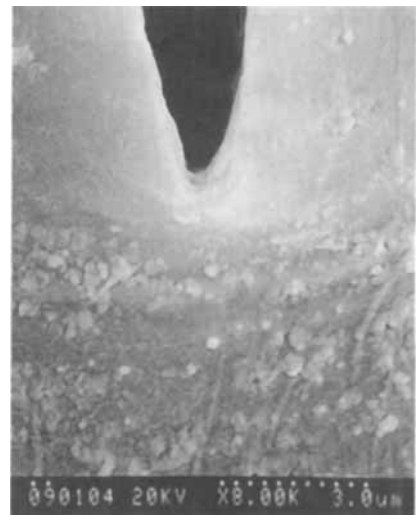
Fig. 6. Crack tip blunting for PC + 2.5% elastomer at point A in Fig. 5.
