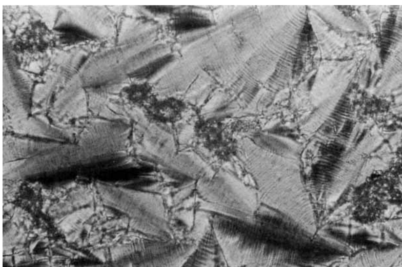
Figure 3. Optical polarized micrographs displayed by polymer VIIIIP (400 \times ): (A) focal-conic texture of the smectic A phase obtained after cooling to 114.8 ^{\circ} C, (B) arced focal-conic texture of the smectic E phase obtained after cooling to 63.7 ^{\circ} C.
