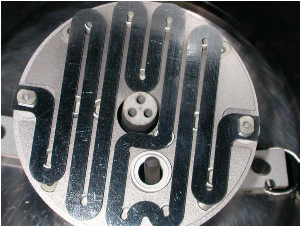
Figure 2-8 Picture of Filament used in EMCORE D-75
