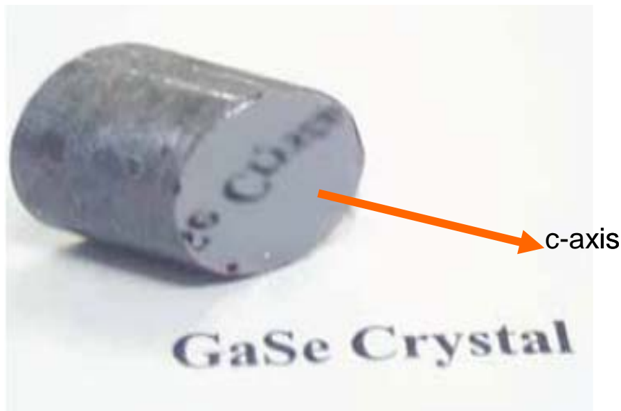
Fig. 1-3 A cleaved surface of the as-grown \epsilon -GaSe crystal.
