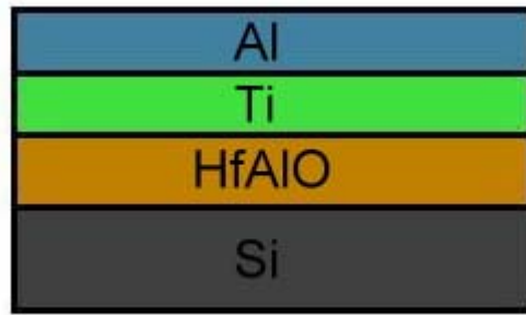
Fig.2-6 400 nm Al was deposited on the Ti layer as top electrode by thermal evaporation coater.
