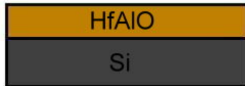
Fig.2-3 (1)Si substrate RCA clean (2)6 nm HfAlO was deposited on the sub-Si by MOCVD.
