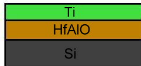
Fig.2-5 40 nm Ti was deposited on the HfAlO layer by dual e-gun evaporation system .
