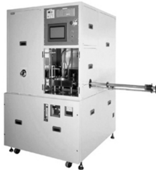
Fig. 4.2. Schematic illustration and photo of the ICP etch system.
