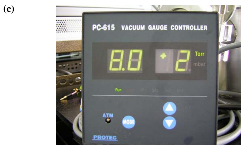
Figure 3.2 (a) The mass flow controller of gas sensing system. (b) The power supply of mass flow controller. (c) The pressure gauge of gas sensing system.
