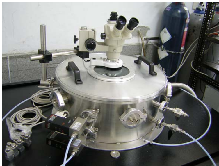
Figure 3.4 Top-view image of gas-sensing system mounting a metal cap with transparent window.
