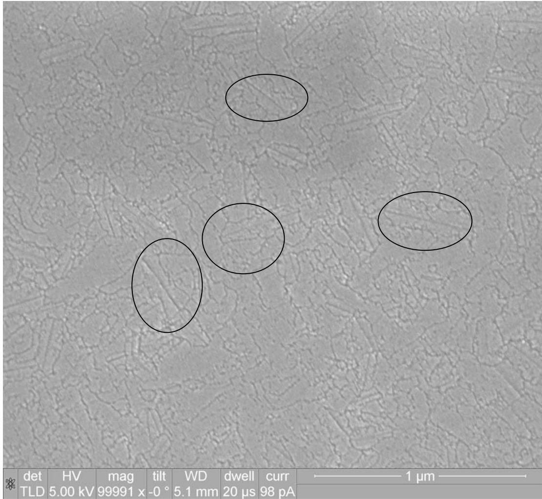
Fig. 3-15(c) SEM pictures of the C-MT channel regions in BE1-3
