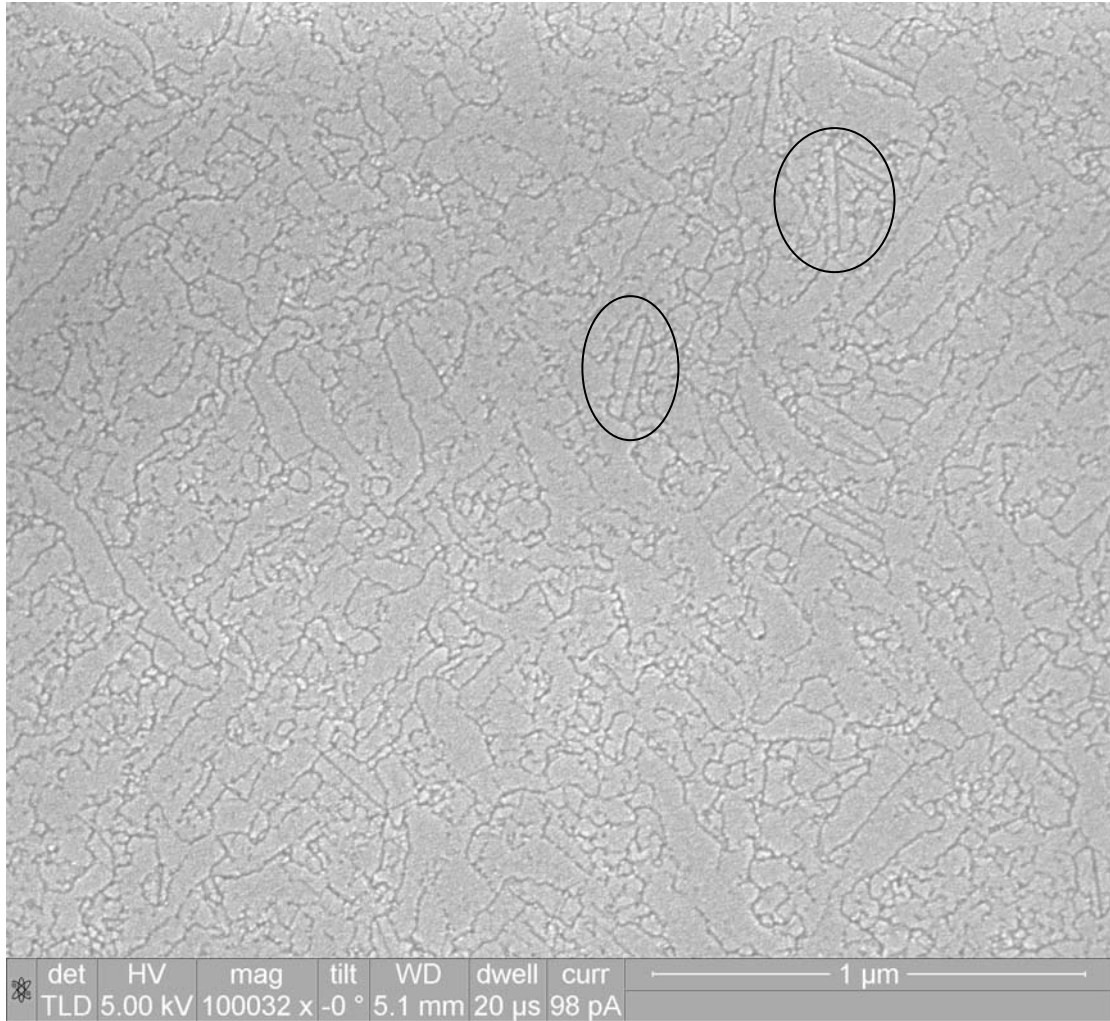
Fig. 3-15(b) SEM pictures of the C-MT channel regions in BE1-2
