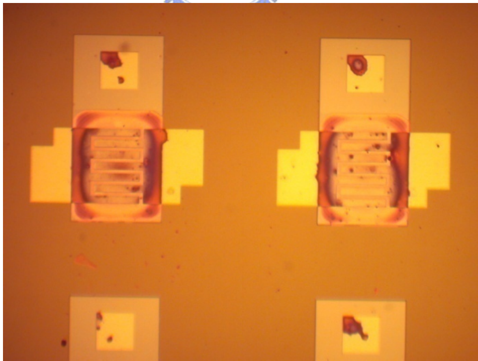
Fig. 3-14 The OM image of PECVD ( \text{SiH}_4 + \text{N}_2\text{O} @ 300\text{ }^\circ\text{C} ) oxide thickness with 100nm.
