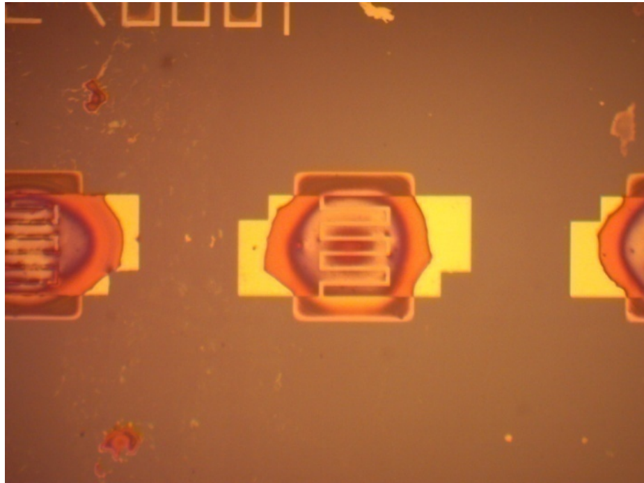
Fig. 3-17 The OM image of Thermal (TEOS@700°C) oxide thickness of 100nm.
