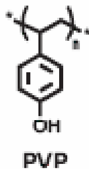
Fig. 2-17 Poly (4-vinylphenol) (PVP) is one of the most popular gate materials.
