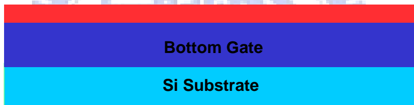
Fig. 2-2 (a) Deposition of in-situ doped n+ poly-Si bottom gate and bottom gate oxide.
