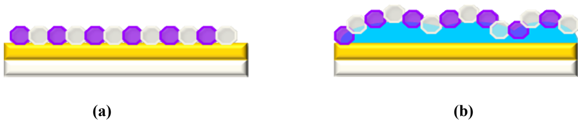
Figure 2-12 The catalyst after pretreatment (a) without Al buffer layer (b) with Al buffer layer.
