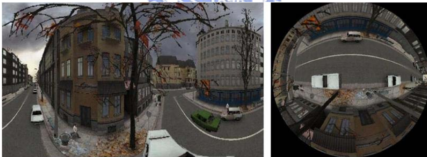
Figure 2-18 The synthetic frames of omnicams: panoramic (left) parabolic catadioptric (right) omni-directional cameras [19]
