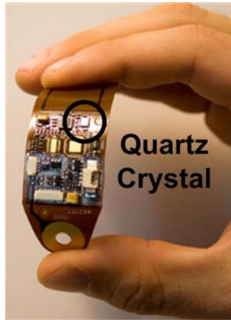
Figure 1-2: The Quartz crystal used in a wireless electrocardiogram (ECG) patch
