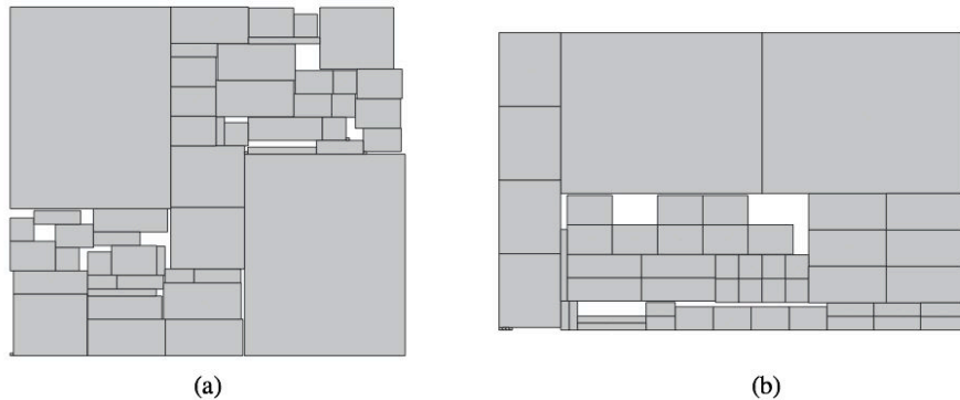
Figure 1.1: (b) describes a structured placement. Compared with (a), we can see that the structured placement groups cells with equal height and width together to make each cluster more rectangular.
