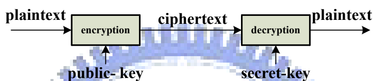
Figure 1.2: Asymmetric-key cryptography block diagram
