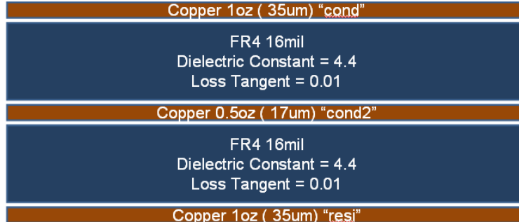
Figure 4.3 The layer stack on PCB
