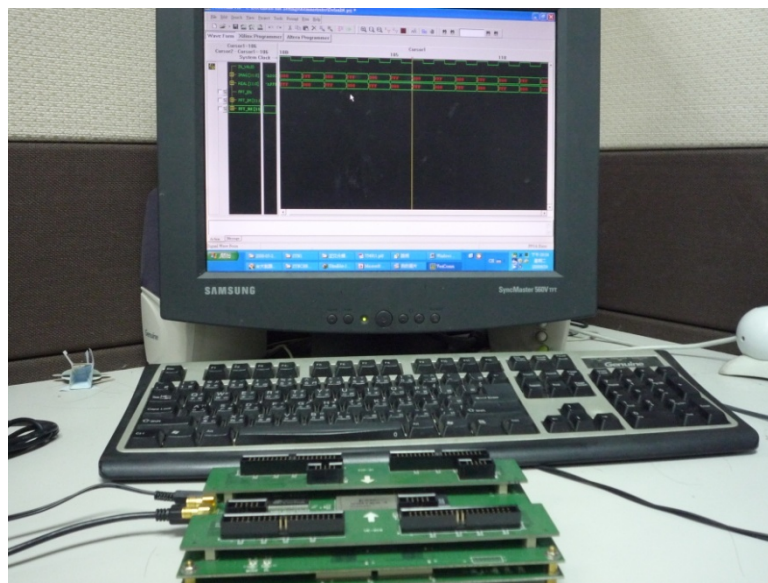
Figure 4.10 VeriComm Pro software and the Xilinx FPGA
