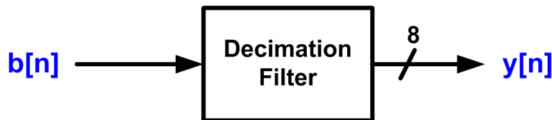
Figure 3.1 Diagram shows the input/output variables of the decimation filter.
