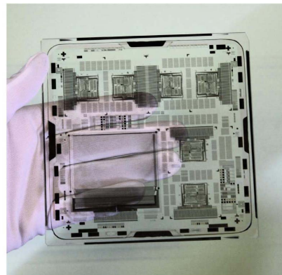
Figure 1.3 (a) The schematic illustration of the “sheet computer” concept and (b) a CPU with an instruction set of 1-4 bytes and an 8-bit data bus on glass substrate.
