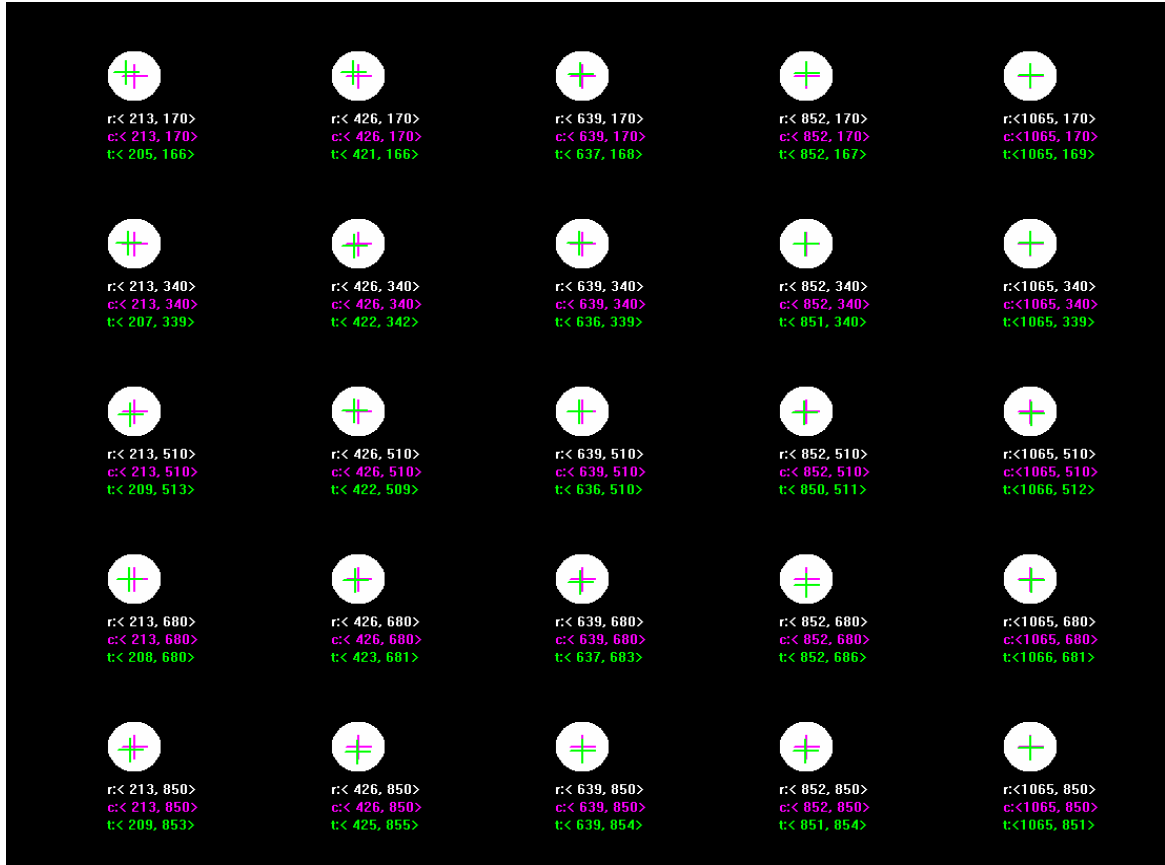
Fig. 5.13 Comparison using calibration image points. The precise landmark position, the computed position by proposed method, and that by Tsai's method are listed under each dot.
