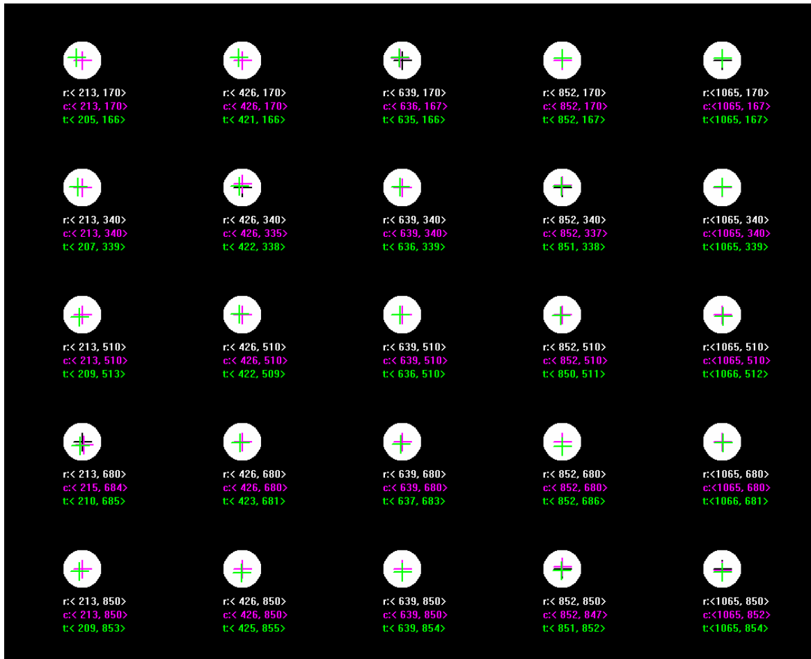
Fig. 5.14 Comparison using re-captured image points. The precise landmark position, the computed position by proposed method, and that by Tsai's method are listed under each dot.
