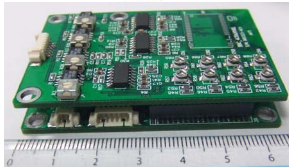
Fig. 3-3: Photo of portable front-end system
