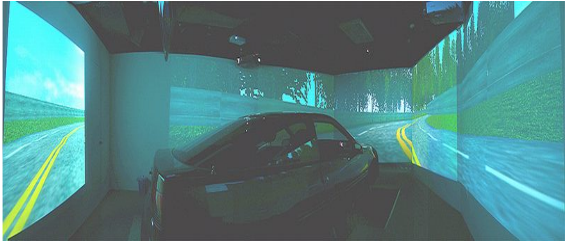
Fig. 5-1: Overview of surrounded VR scene. The VR-based four-lane highway scenes are projected into surround screen with seven projectors processing.
