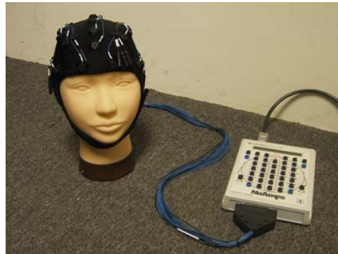
Fig. 2-3: Photo showed the setup of the physiological recording containing the NuAmps EEG amplifier and the electrode cap.
