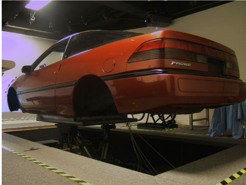
Figure 2: A car body mounted on a 6-DOF Stewart motion platform.
