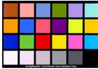
Fig. 4.11 GretagMacbeth™ ColorChecker Color Rendition Chart (each block is mark as 1 to 24, from the left-to-right, and top-to-bottom)
