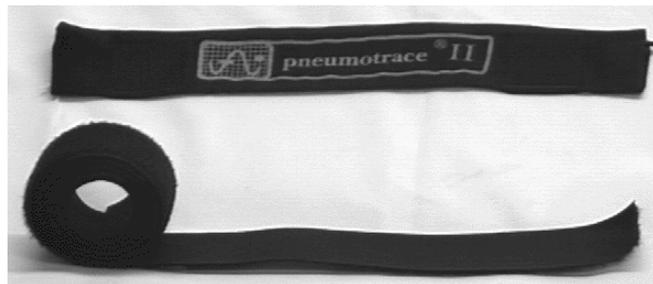
Fig. 3.4. Piezo-electric respiratory transducer.
