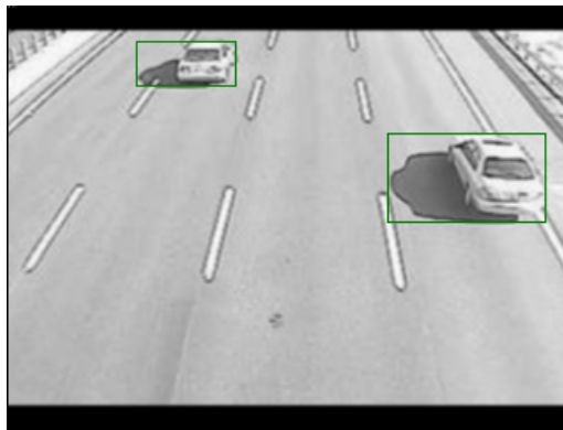
Fig. 3-10: Moving Object with minimum bounding rectangle
