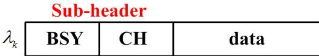
Fig. 14: Packet format of IWS
