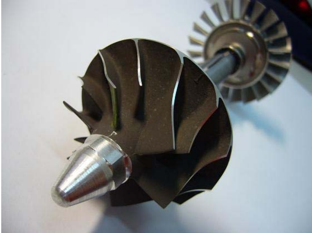
Fig. 2-6 the picture of compressor
