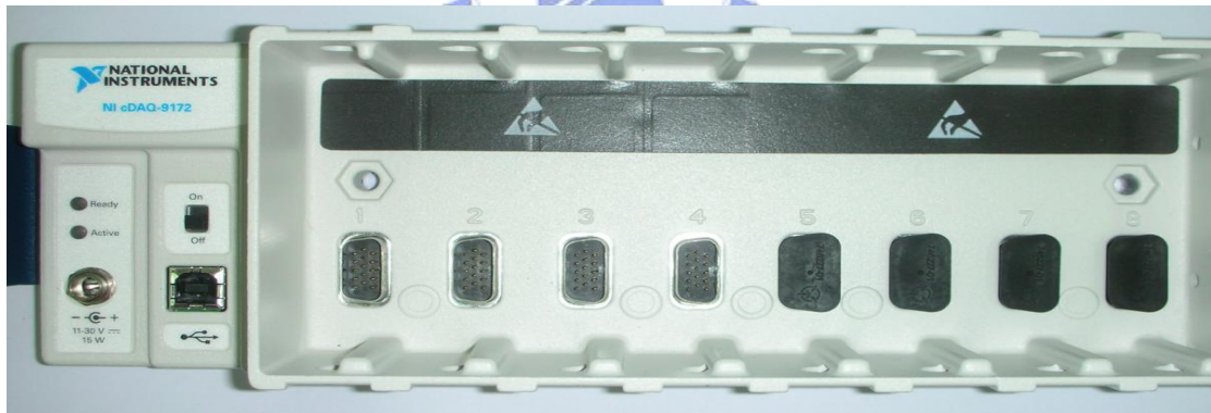
Fig. 2-18a The CompactDAQ Chassis
