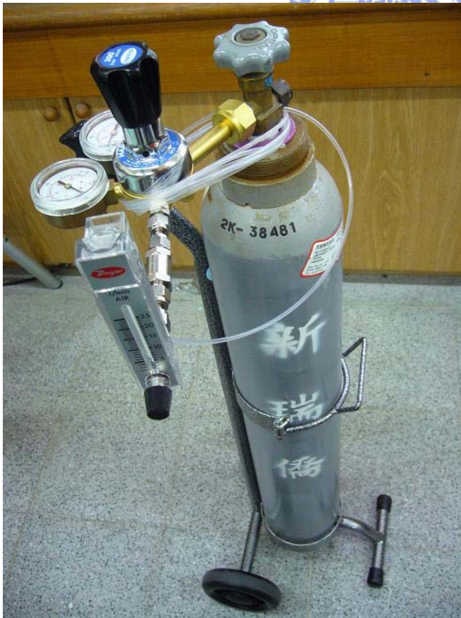
Fig. 2-10 Methane bottle & pressure valve & flow meter
