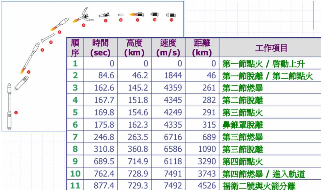
**Fig.1.1** The flying diagram of Formosat-2
