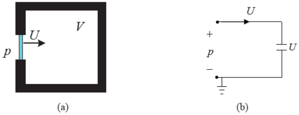
Figure 5. (a) Closed volume of air that acts as acoustic compliance. (b) Analogous circuit.
