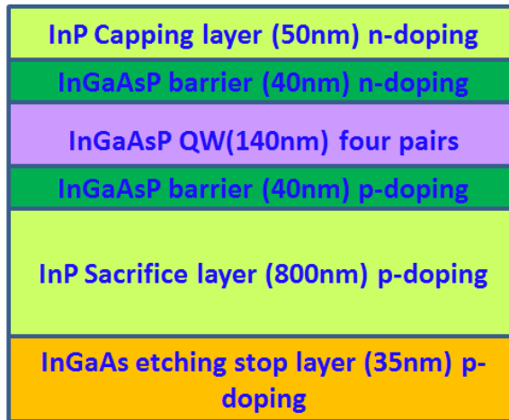
Fig. 3. 1: The epitaxial structure of doped InGaAsP MQWs for electrical driving by central post.
