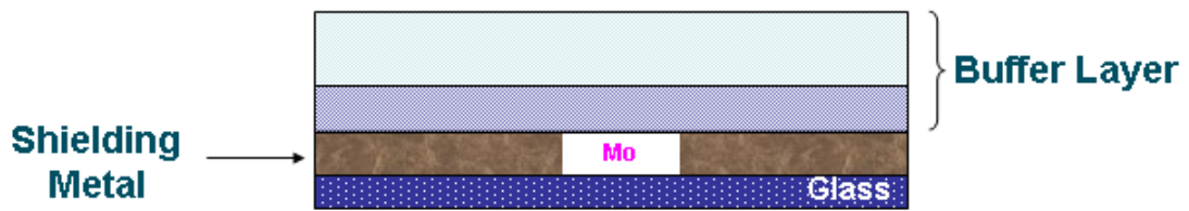
Fig.2.2.1 Structure of shielding metal which was employed Molybdenum.
