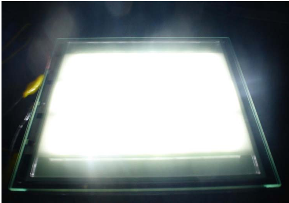
Fig. 4-6. The optical appearance of the CPL filled with 50 torr, pure xenon gas, under the frequency 50 kHz, current 0.13 A and voltage 260 V.
