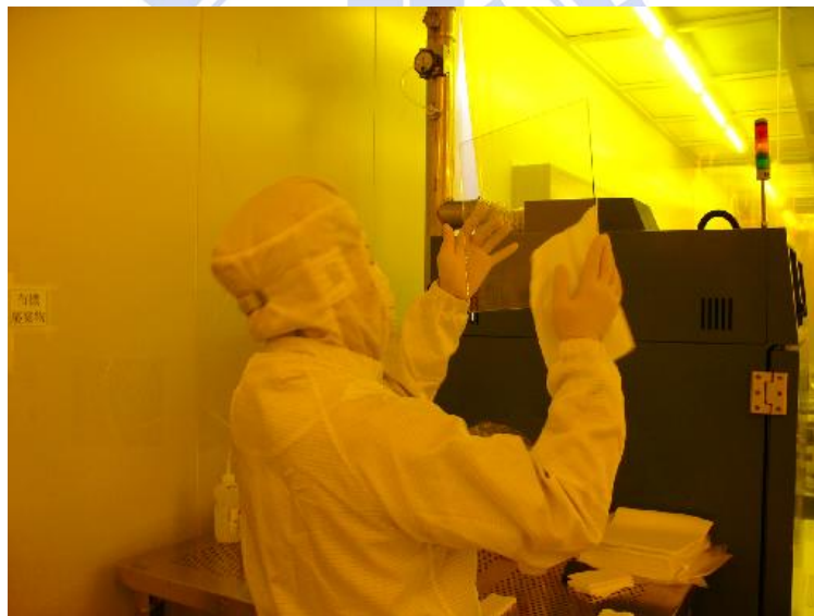
Fig. 3-3. The glass substrate cleaning before all the processes.
