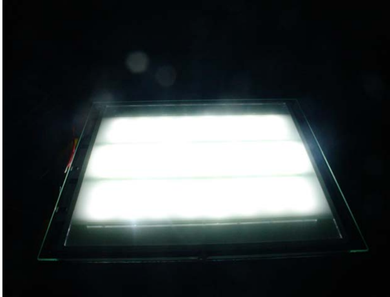
Fig. 4-1. The optical appearance of NTL filled with 50 torr, pure xenon gas, under the frequency 50 kHz, current 0.26 A and voltage 260 V.
