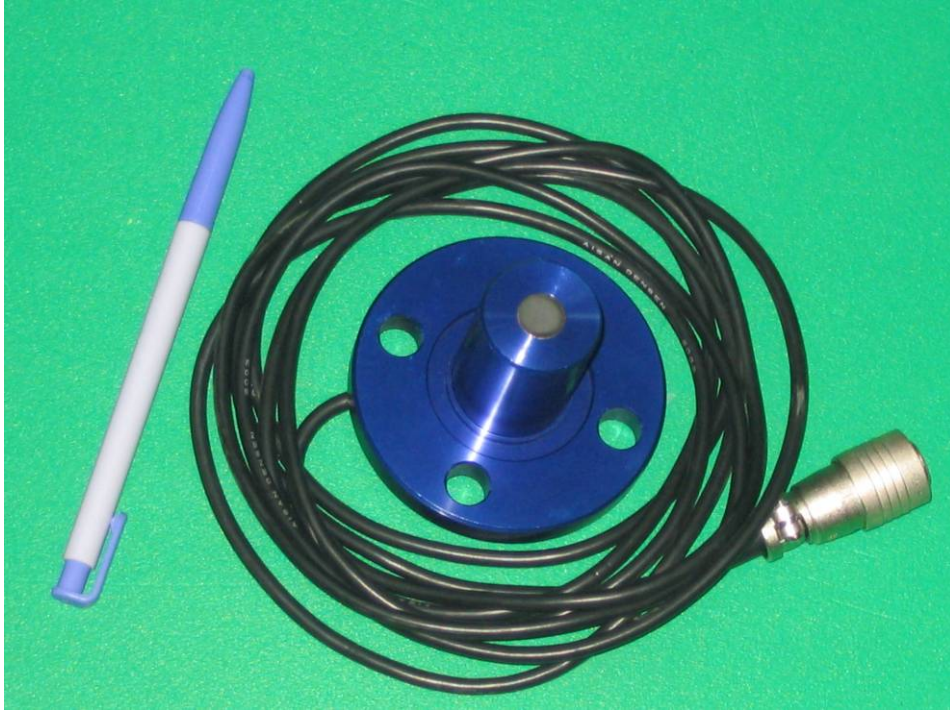
Fig. 3.5. Soil pressure transducer (Kyowa PGM-0.2KG)
