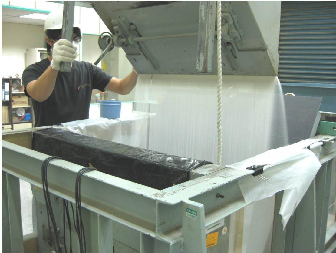
Fig. 5.14 Pluvion of Ottawa sand into soil bin
