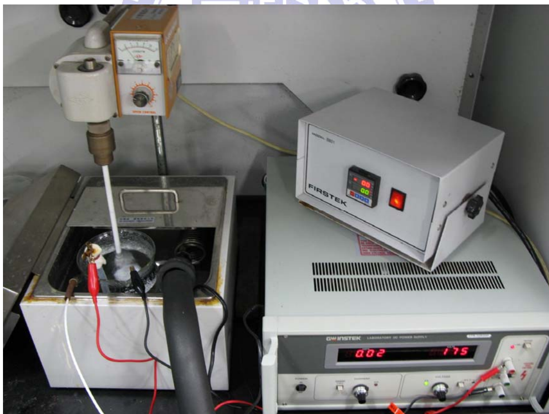
Figure 3.2. A schematic diagram and practical cell picture of the experimental fixtures used to fabricate AAO specimens.
