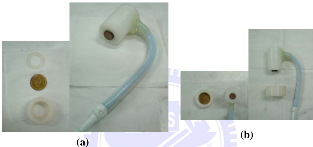
Fig.3-7 The samples of electro-polishing. (a) The front view of holder and it had a conductive piece of Cu. (b) The holder were used to put the indium in it.
