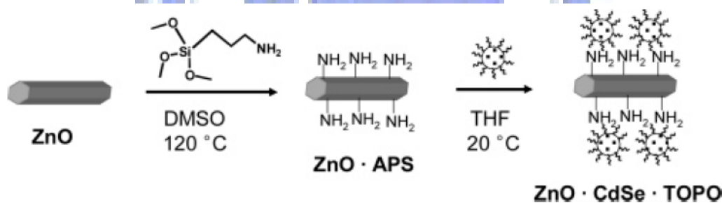
Figure 1-2-2. Unidirectional light emitters were synthesized from rod-shaped ZnO microcrystals and TOPO coated CdSe/CdS core/shell nanoparticles.
