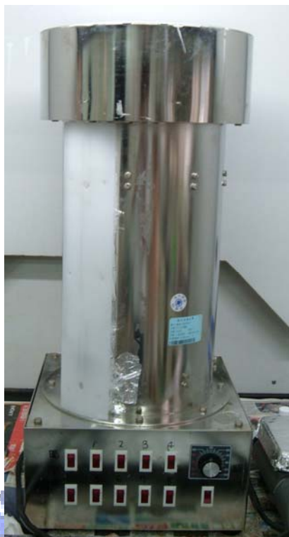
Figure 3- 4 Photoreactor and the wavelength of UV-lamp is 305 nm in our study.
