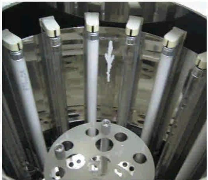
Figure 3-9 A design chart for photocatalysis reactor and A photograph of photocatalytic reactor.
