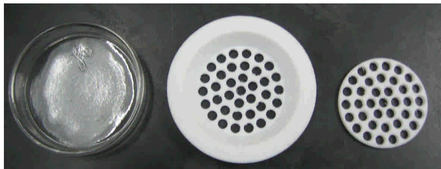
Figure 3-5 A design chart and a photograph of surface sol-gel system.
