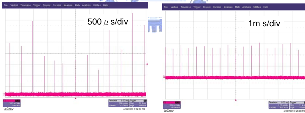
Fig.5.15. The improvement of the stability of the pulse train. Left: the PQS pulse train; right: the hybrid Q-switched pulse train.
