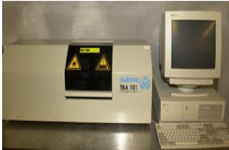
Fig. 3-5 Pretilt angle measurement system (Autronic DMS 101 TBA)
