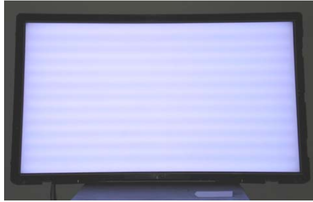
Fig. 1-4 Lamp-Mura defect of a 32-inch direct-emitting backlight system captured by a charge-coupled device (CCD).
