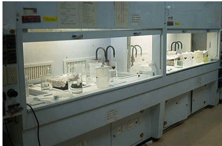
Fig.2-1. Photograph of Wet Bench.
