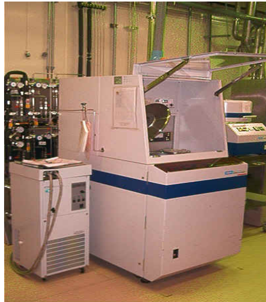
Fig.2-4 . Photograph of Reactive Ion Etching System.
