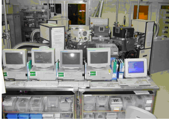
Fig.2-2. Photograph of PECVD system.
