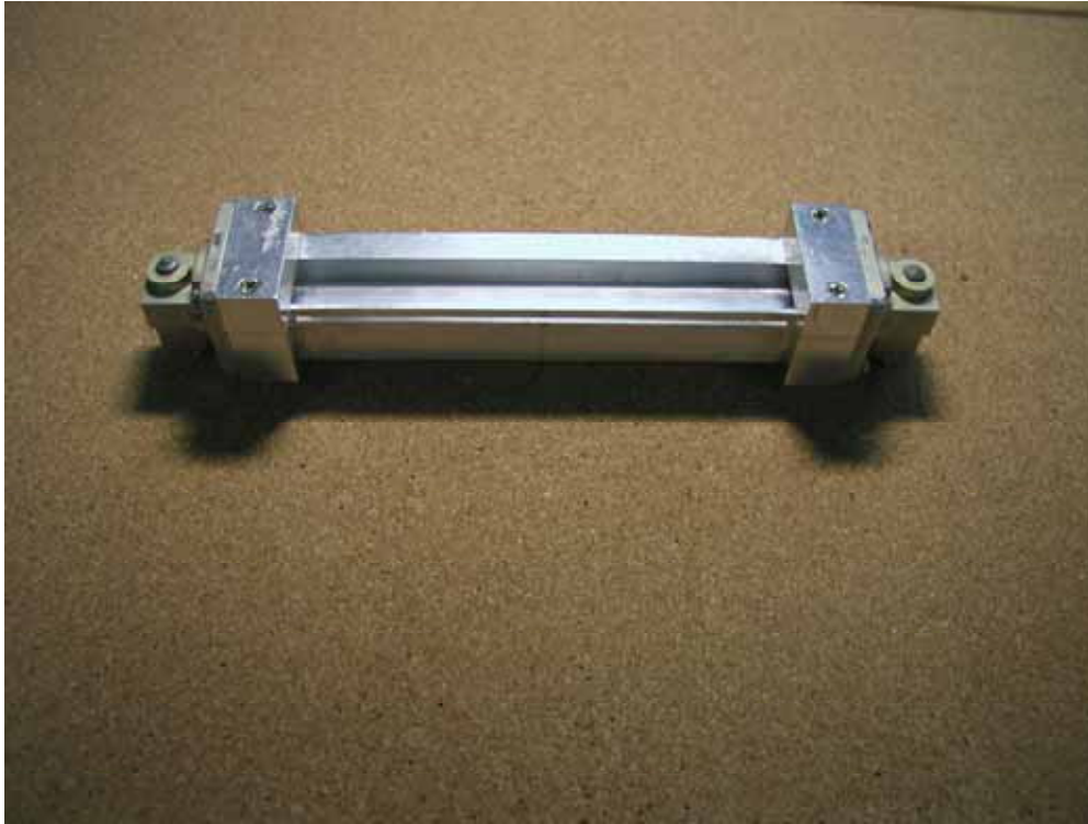
Figure 3(d) A slitted waveguide with input and output ports.
