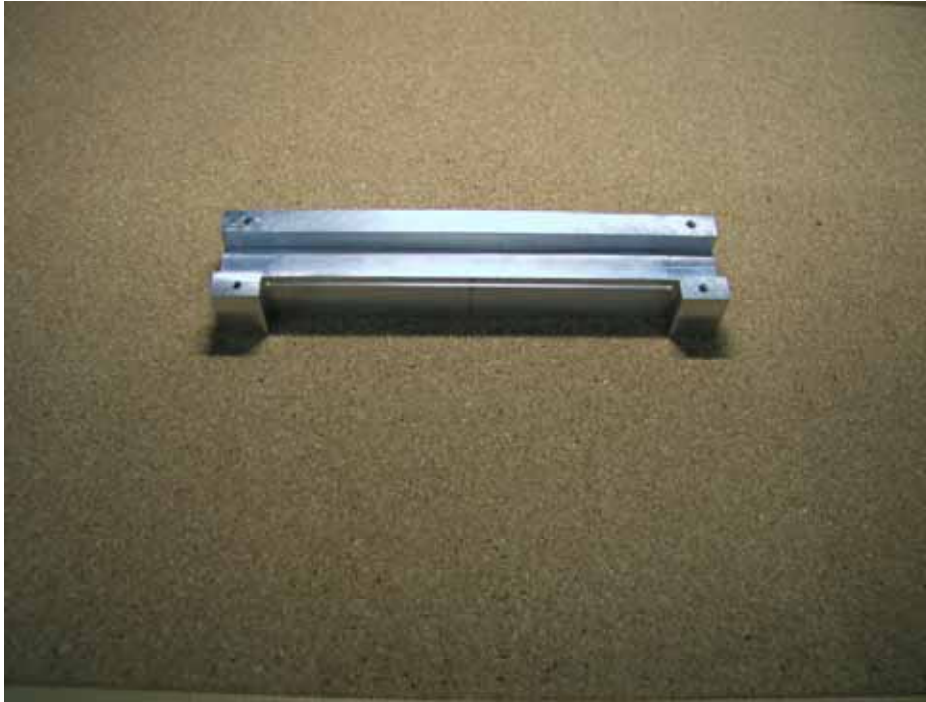
Figure 3(b) A slitted waveguide with bottom plate removed.
