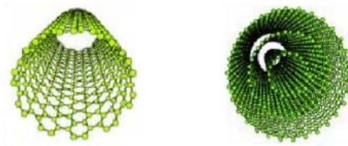
Figure 2.4 Schematic diagram of (a) a SWNT and (b) a MWNT
